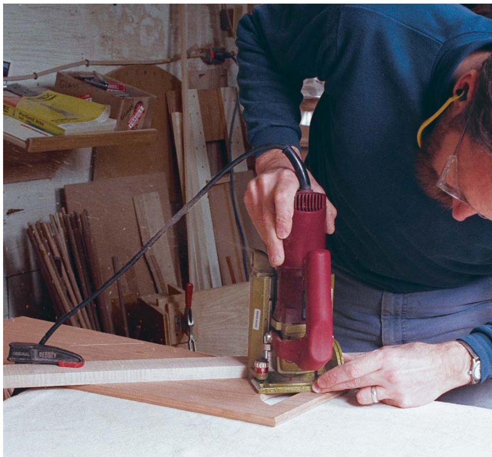
A straight board guides the biscuit joiner. The author places the base of the tool against a board clamped to the side to cut the slots for the shelves.
